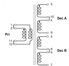
Primary:  $L = 194 \mu H$ DCR =  $0.015\Omega$ Irms = 5.8 AVT = 131.9 V- $\mu$ sec Each half secondary; Sec A (3-9), Sec B5-7): DCR =  $0.06\Omega$ Irms = 2.9 A
