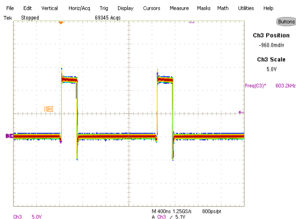
Fig. 21. Inductor node at 8A load Ch3: LX
