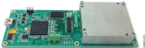
Figure 2. ADIS16488 Installation Example
