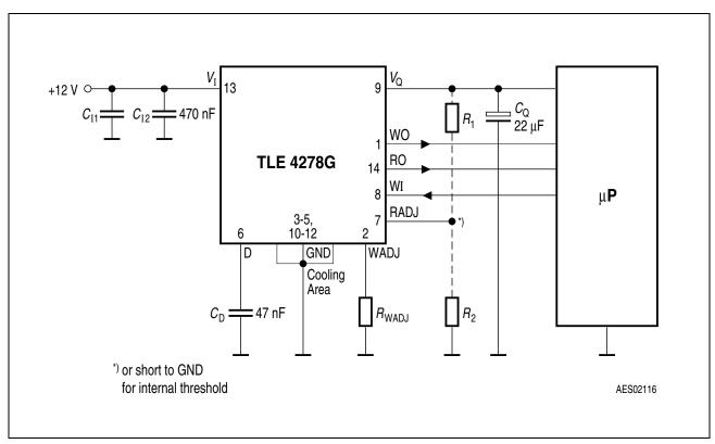
Figure 4 Application Circuit
