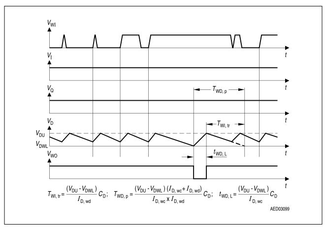
Figure 8 Timing of the Watchdog Function
