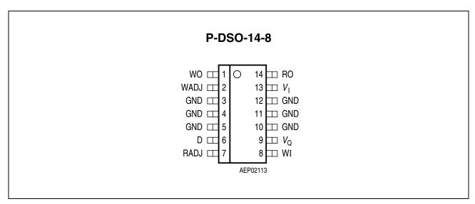
Figure 1 Pin Configuration (top view)
