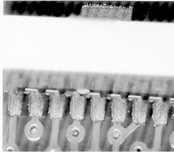
Photo 1.0. Castellation misaligned to land pads in x-axis before reflow.
