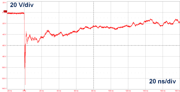
Figure 8. Response to ISO 10605 -C = 150 pF, R = 330 Ω (-8 kV contact)
