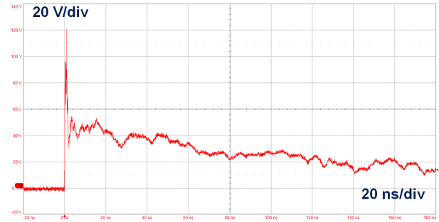
Figure 9. Response to ISO 10605 - C = 150 pF, R = 330 Ω (+8 kV contact )
