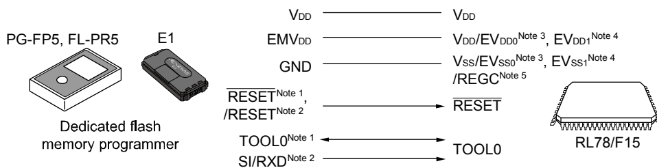
Figure 31-2. Communication with Dedicated Flash Memory Programmer
