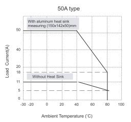
Max. load Current vs. Ambient Temp.
