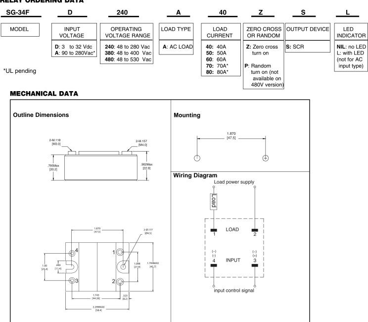
Dimensions in inches with metric equivalents in parentheses. Tolerance: ± .010"
