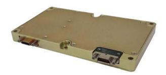
The RF-7850A-PS001 is a very low-profile, ruggedized solution supporting deployment of the RF-7850A-UA Unmanned Aircraft Networking Radio in platforms using MIL-STD-704 compliant VDC power. This high-efficiency DC/DC-mounted power supply converts 28 VDC to 12 VDC for the UA. It includes EMI filters, input/output isolation capabilities, zero voltage switching technology and over-voltage and over-temperature shutdowns with auto recovery.
