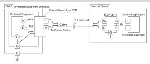
Connect the MD6T's green leadwire to the ground terminal inside the protected equipment enclosure to ground through the enclosure's outside ground terminal.
