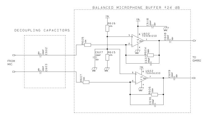
This circuit has a gain of 15 times (+24 dB), and is therefore suited for the internal mic. input, having a microphone with a sensitivity close to the suggested one (-45 dB<sub>Vrms/Pa</sub>), if the used microphone has a different sensitivity, or if the buffer is connected to the external mic. input, then a gain adjustment shall be done by changing resistors R604-R605 and R606-R607 and as a consequence the capacitors C636 and C637 to maintain the bandwidth 150-8000 (-3dB).
