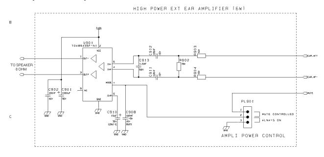
An example of car kit amplifier schematic can be:
