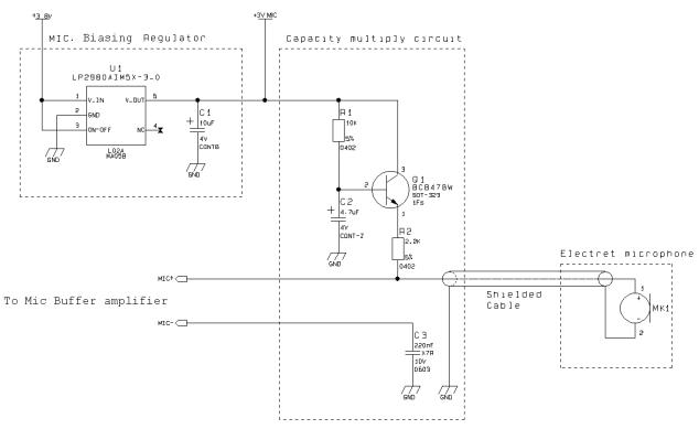
For example a circuit for the unbalanced microphone biasing can be:
