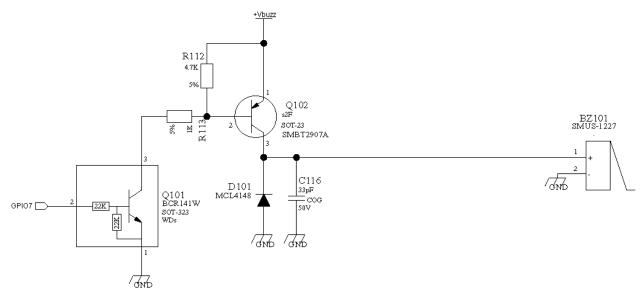
NOTE: To correctly drive a buzzer a driver must be provided, its characteristics depend on the Buzzer and for them refer to your buzzer vendor.
