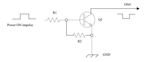
**NOTE:** don't use any pull up resistor on the ON# line, it is internally pulled up. Using pull up resistor may bring to latch up problems on the GE863-QUAD power regulator and improper power on/off of the module. The line ON# must be connected only in open collector configuration.
