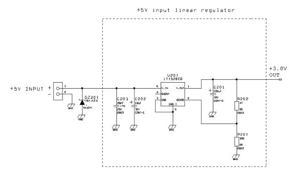
An example of linear regulator with 5V input is:
