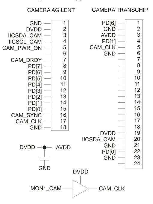
The numbers on the left side of the Camera's connectors refers to Module Connector's pin number.
