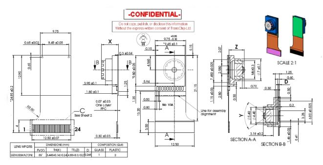
Fig 1. Camera Physical Detail & Connector
