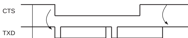
Figure 36-28. Transmitter Behavior when Operating with Hardware Handshaking
