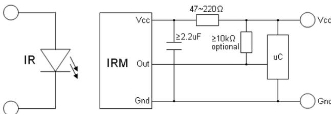
The RC Filter must be connected as close as possible to  $V_{CC}$  and GND pins.
