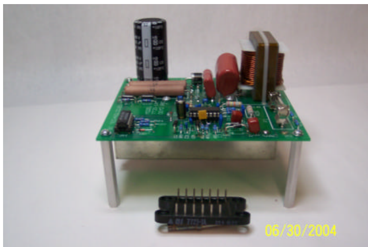
The 7720-1-EVM Evaluation Board is a working example of a complete PFC front end for power supplies from 500watts to 2500 watts. The circuit is based on BI's 7720-1A power module, which contains all of the power semiconductors for this application. It is attached on the underside of the evaluation board.
