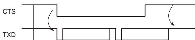
Figure 36-28. Transmitter Behavior when Operating with Hardware Handshaking
