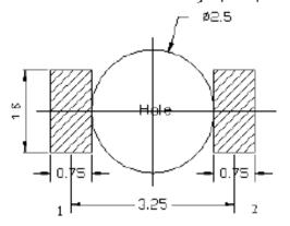
Note: Tolerances unless mentioned ±0.1mm. Unit = mm Suggested pad dimension is just for reference only. Please modify the pad dimension based on individual need.
