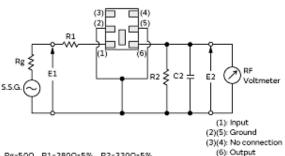
Rg=50Ω R1=280Ω±5% R2=330Ω±5% C2=10±2pF (Including stray capacitance and Input capacitance of RF voltmeter) E1: S.S.G. Output Voltage
