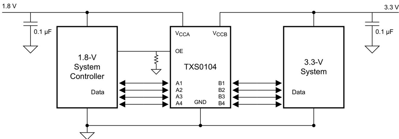
Figure 11. Application Schematic
