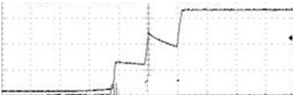
Figure 20. Supply Voltage Drop
