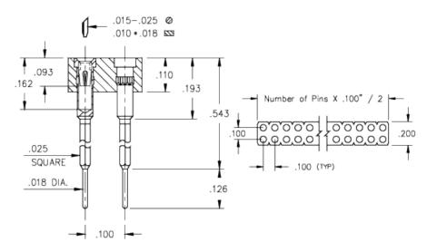
**Description:** Interconnect Socket Wrapost with Solder Tail Socket Accepts .015"- .025" (0,38 - 0,635 mm) dia leads Double Row Through Hole Plating Code: Shell Plating:
