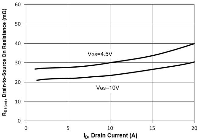
Fig. 4 On-Resistance vs. Gate to Source
