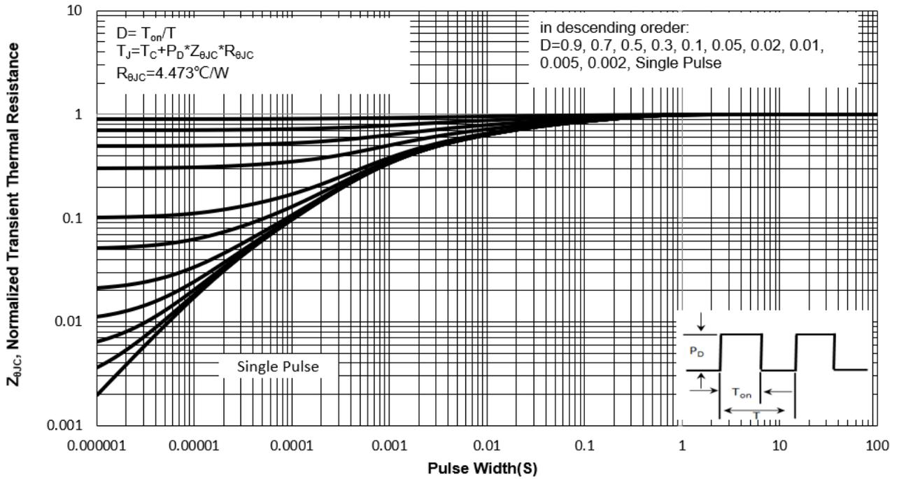
Fig.14 Normalized Maximum Transient Thermal Impedance( $Z_{\theta JA}$ )
