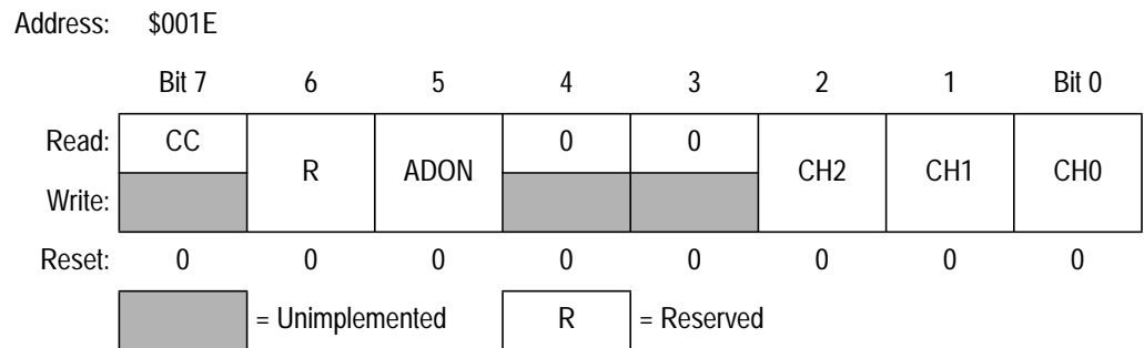
Figure 9-1. A/D Status and Control Register (ADSC)
