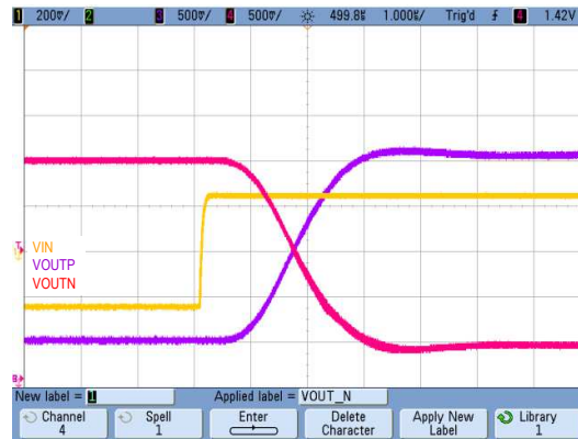
Figure 53. Step Response of the AMC1300
