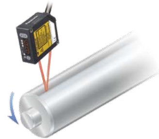
Measuring the eccentricity of a metal shaft
