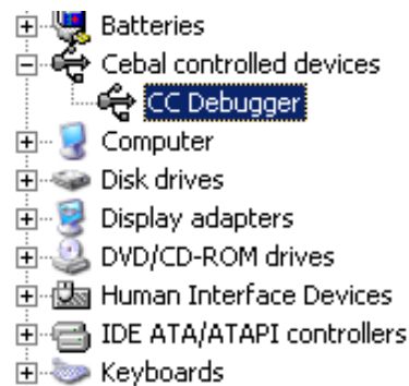
Figure 1. Verify Correct Driver Installation
