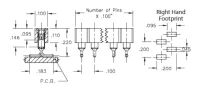
**Description:** Interconnect Socket Surface Mount Socket Accepts .015" - .025" (0,38 - 0,635 mm) dia leads Single Row Surface Mount **Plating Code: Shell Plating:** 200 μ" Tin/Lead(93/7) over 100 μ" Nickel
