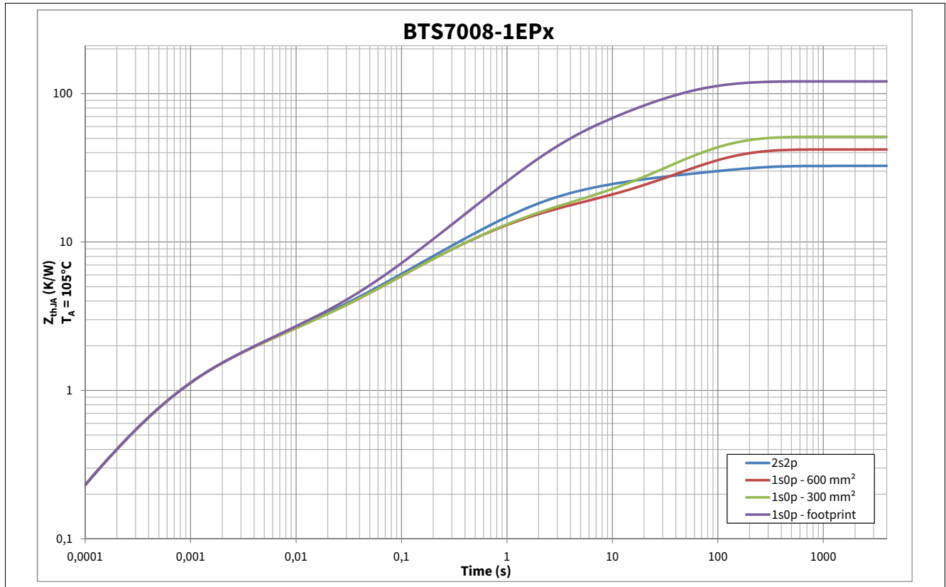
Figure 9 Typical Thermal Impedance. PCB setup according Chapter 4.4.1
