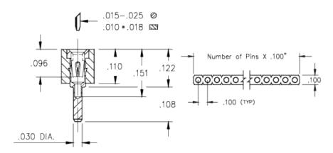
**Description:** Interconnect Socket Low Profile Solder Tail Socket Accepts .015" - .025" (0,38 - 0,635 mm) dia leads Single Row Through Hole Plating Code:
