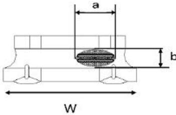
Appearance of exposed wire tolerance limit:
