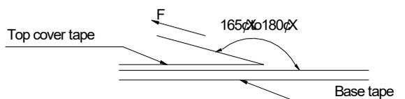
The force for tearing off cover tape is 15 to 80 grams in the arrow direction under the following conditions.
