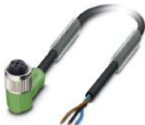
Sensor/actuator cable, 3-position, PUR halogen-free, black-gray RAL 7021, free cable end, on Socket angled M12, coding: A, PIN 2+4 bridged, cable length: 5 m
