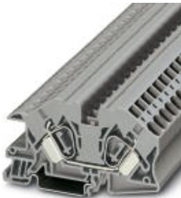
Installation level terminal block, Spring-cage connection, Cross section: 0.2 mm 2 - 16 mm 2 , AWG: 24 - 6, Width: 10 mm, Color: blue, Mounting type: NS 35/7,5, NS 35/15
