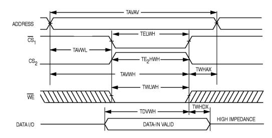
Note: The internal write time of the memory is defined by the overlap of  $\overline{CS1}$  Low and CS2 HIGH and  $\overline{W}$  LOW. Both signals must be actived to initiate a write and either signal can terminate a write by going in actived. The data input setup and hold timing should be referenced to the actived edge of the signal that terminates the write. Data out is high impedance if  $\overline{OE} = V_{H}$ .
