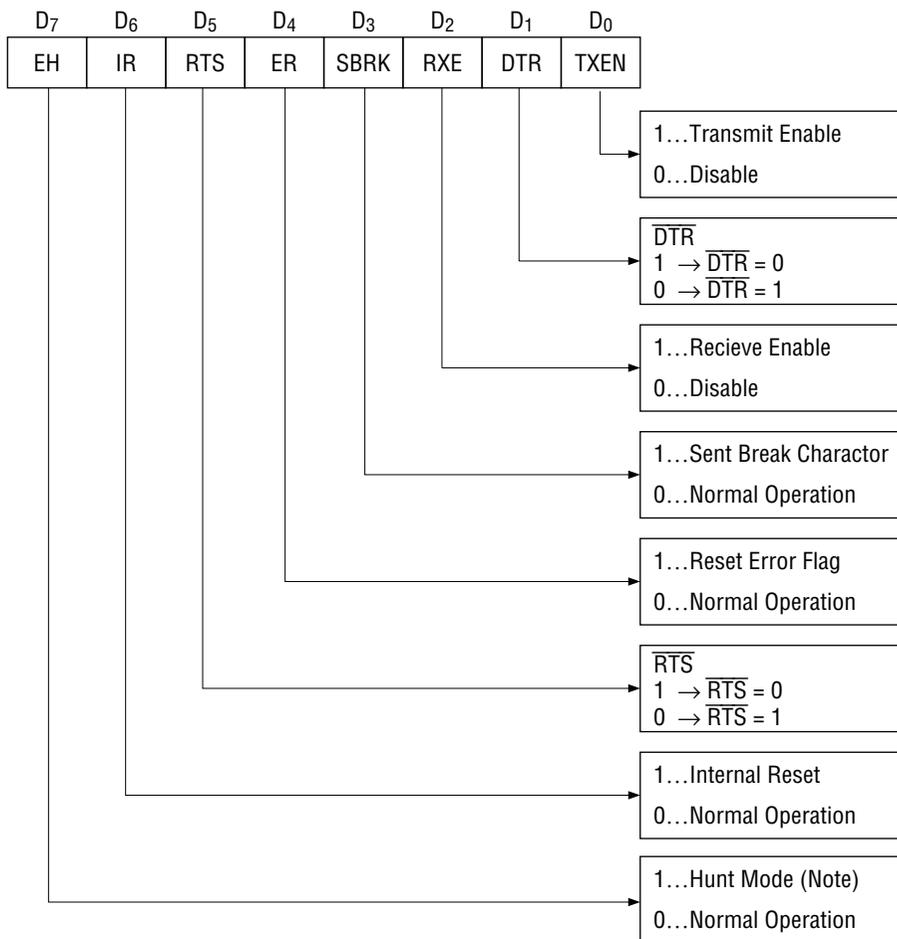
**Note:** Seach mode for synchronous characters in synchronous mode.
