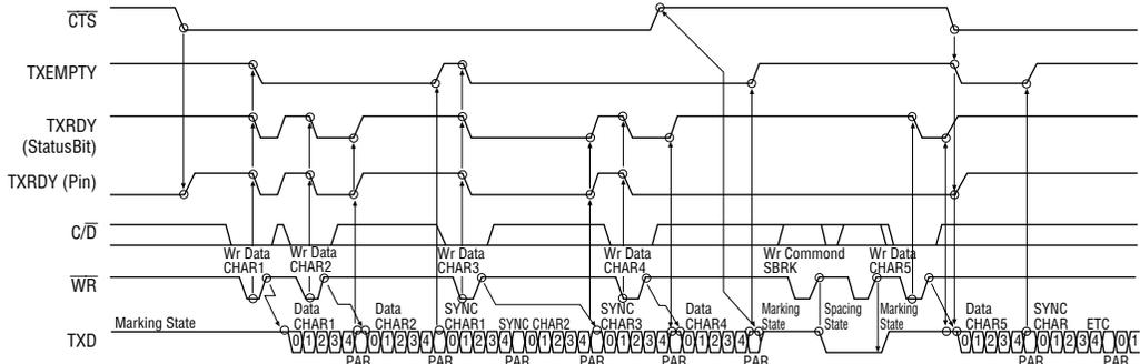
**Note:** The wave-form chart is based on the case of 5 data bit length + parity bit and 2 synchronous characters.
