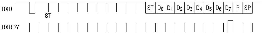
A RXRDY signal is outputted during data reception due to a malfunction.
