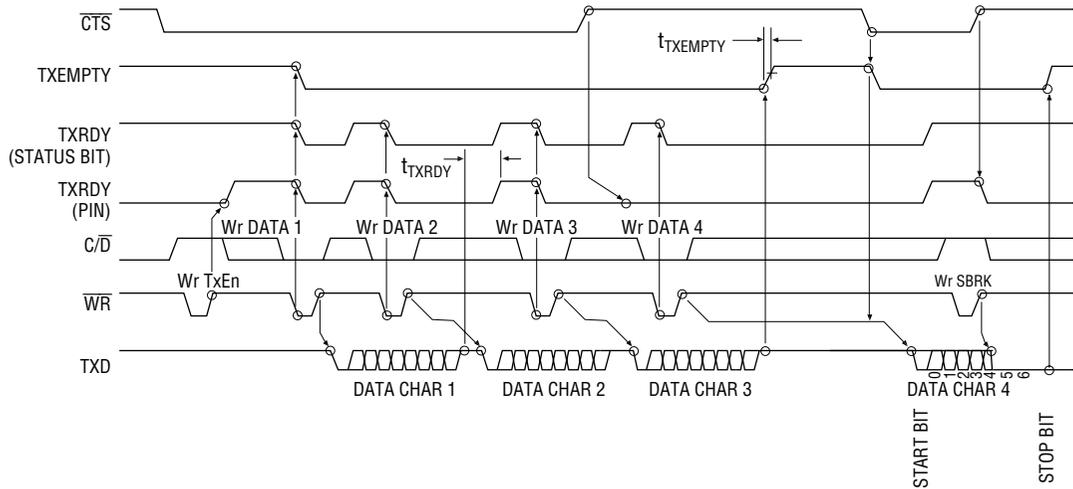
**Note:** The wave-form chart is based on the case of 7-bit data length + parity bit + 2 stop bit.
