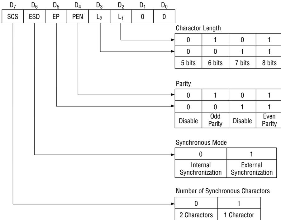
**Fig. 3 Bit Configuration of Mode Instruction (Synchronous)**
