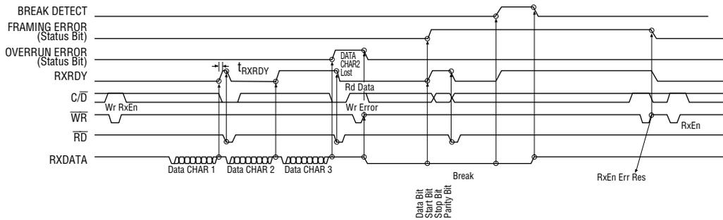
**Note:** The wave-form chart is based on the case of 7 data bit length + parity bit + 2 stop bit.
