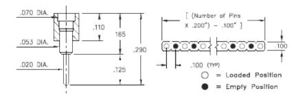
Interconnect Socket Standard Solder Tail Socket Accepts .015"- .025" (0,38 - 0,635 mm) dia leads Single Row Through Hole Plating Code: 43 Shell Plating: 200 µ" Tin (matte finish) over 100 µ" Nickel Inner Contact Plating: 30 µ" Gold over 50 µ" Nickel Packaging:
