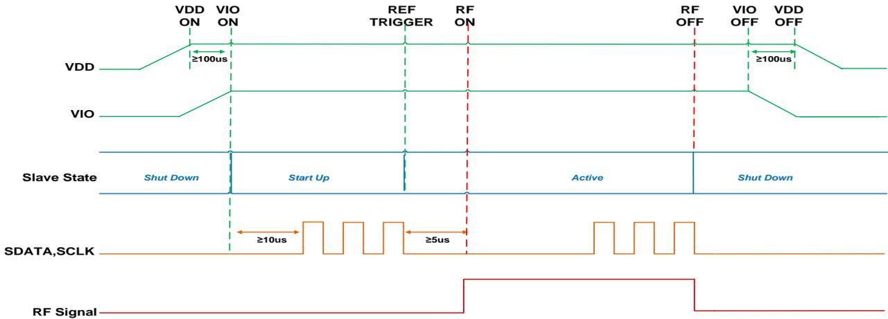
**Note 3:** VIO can be applied to the device after VDD or removed before VDD. It is important to wait 10µs after VIO & VDD are applied before sending SDATA to ensure correction data transmission. The minimum time between a power up and power down sequence (and vice versa) is  $\geq 100\mu\text{s}$ .
