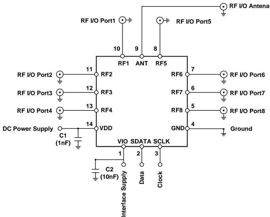
**WS7808QM-14/TR Evaluation Board Schematic**
