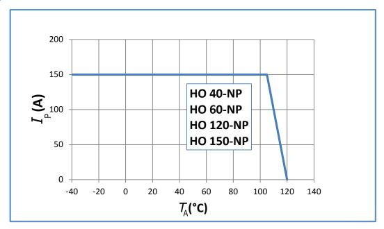
Important notice: whatever the usage and/or application, the transducer jumper temperature shall not go above the maximum rating of 120 °C as stated in page 2 of this datasheet.
