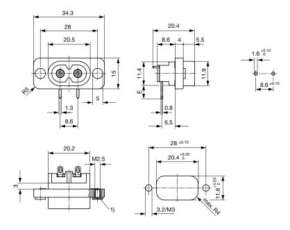
E = PCB terminal standard (additional solder): 6.9 mm
