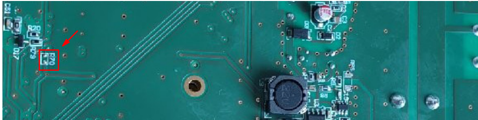
Figure 10. UCB UART Disable via Soldering R70 at MDK Board
