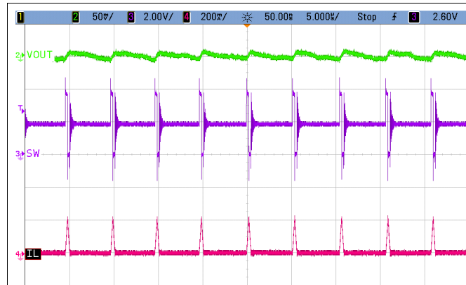
图 20. PFM (Power Save Mode) Mode Operation
