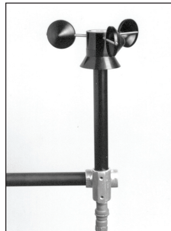
013 Wind Speed Sensor
