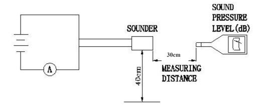
In the measuring test, buzzer is placed as follows:
