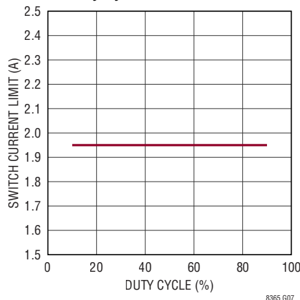
Switch Current Limit vs Duty Cycle
