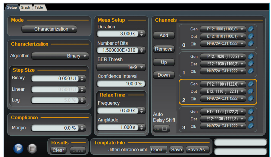
Figure 15. Jitter tolerance setup panel in N4980A.
