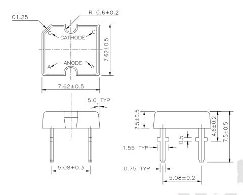
Note: 1. Tolerances unless mentioned  $\pm 0.25$ mm. Unit = mm
