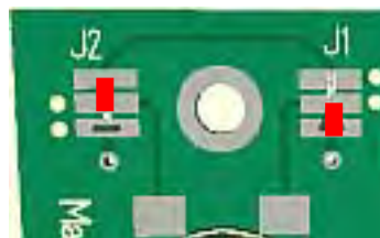
Solders pad J_1 and J_2 connection for reversed heat flux direction
