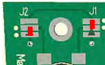
Solder pads J_1 and J_2 connection for heat flux direction (standard delivered)
