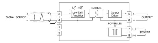
This unit, by its fast-response feature, is not designed to eliminate noise present in the input signal. Use a shielded twisted-pair cable for preventing noise entering through the input wiring.
