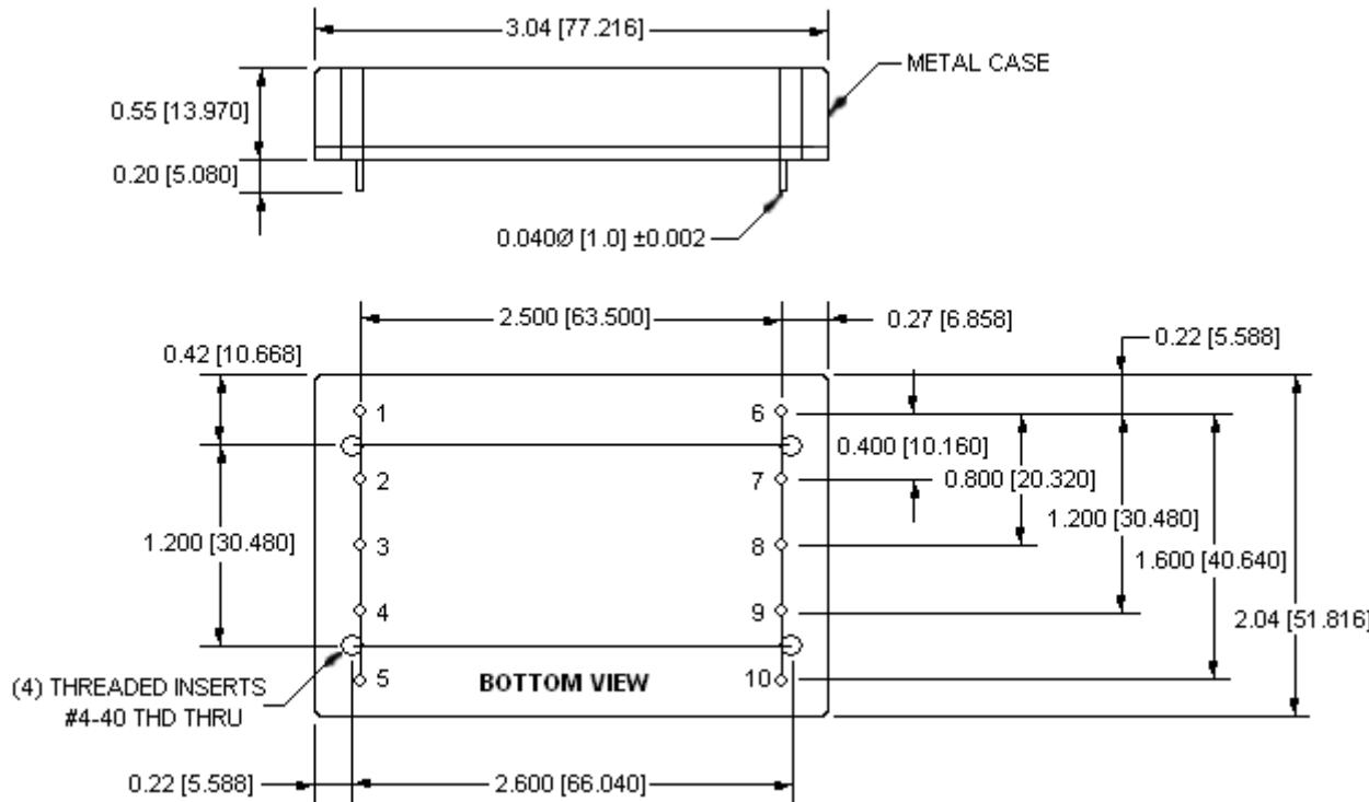
Case and pin-to-case measurements for reference only unless otherwise noted.
