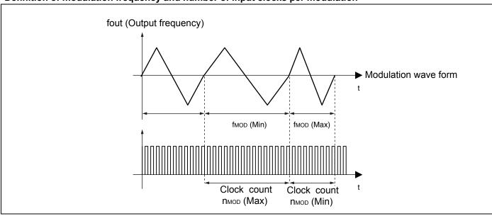
MB88154A contains the modulation period to realize the efficient EMI reduction.
