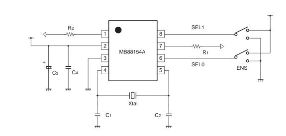
C<sub>1</sub>, C<sub>2</sub> : Oscillation stabilization capacitance (refer to "Oscillation Circuit".)
