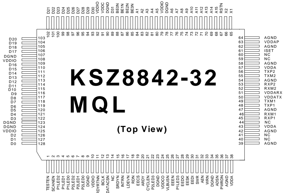
Figure 5. Standard – KSZ8842-32 MQL 128-Pin PQFP (Top View)
