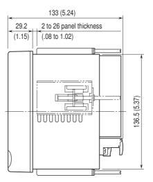
Attach the mounting bracket either on the top/bottom or on the sides.
