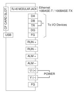
\*Short across these terminals when the device is at the extreme end of a transmission line.
